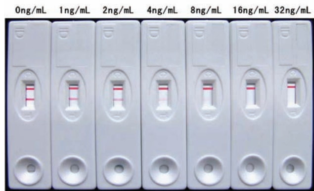
Figure 5. Standard OLA were added in pig urine samples (A) and muscle tissue samples (B) tested using the test strips and the test lines with the naked eye.
